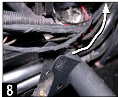
8 Route the harnesses upward behind the center dash where the panel was removed for easier access. Secure with zip ties to factory wiring.
