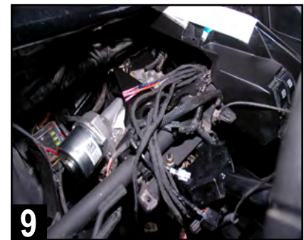
9 Route harnesses up to steering column support bar. Finally, route passenger speaker harness from right speaker location to left harness area.
