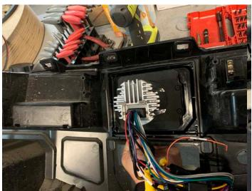
Position rear bracket and loosely install the two nuts on back of radio
