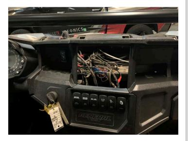
Remove lower switch locations (If your vehicle has switches installed note connections and disconnect)
