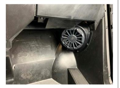
Repeat on the driver side and drill the five lower holes with 11/32" drill bit and secure with five push pins
