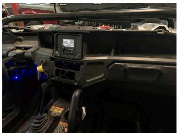
Connect switches, 12-volt accessory port, and connect USB / AUX port to radio then snap center section to dash
